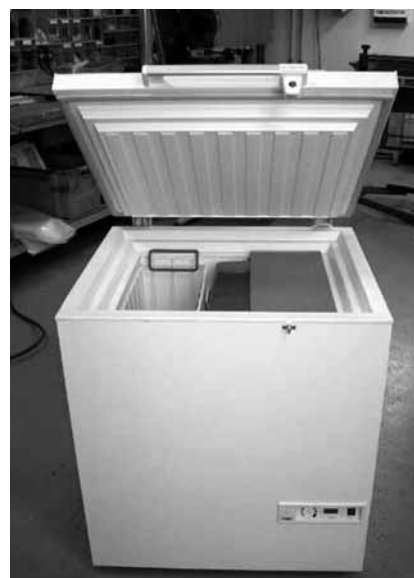
Photo1: Prototype of vaccine cooler. The vaccine will be placed in three baskets, placed vertical in the left side of the cabinet. The ice storage is placed under the blue lid in the right side of the photo. The compressor is placed in a room under the ice storage.
