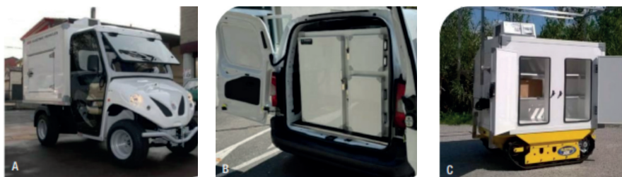
Figure 4: Eutectic solutions: (A) full electric last-mile delivery light vehicle; (B) multi-temperature transport in a van; (C) full electric.
